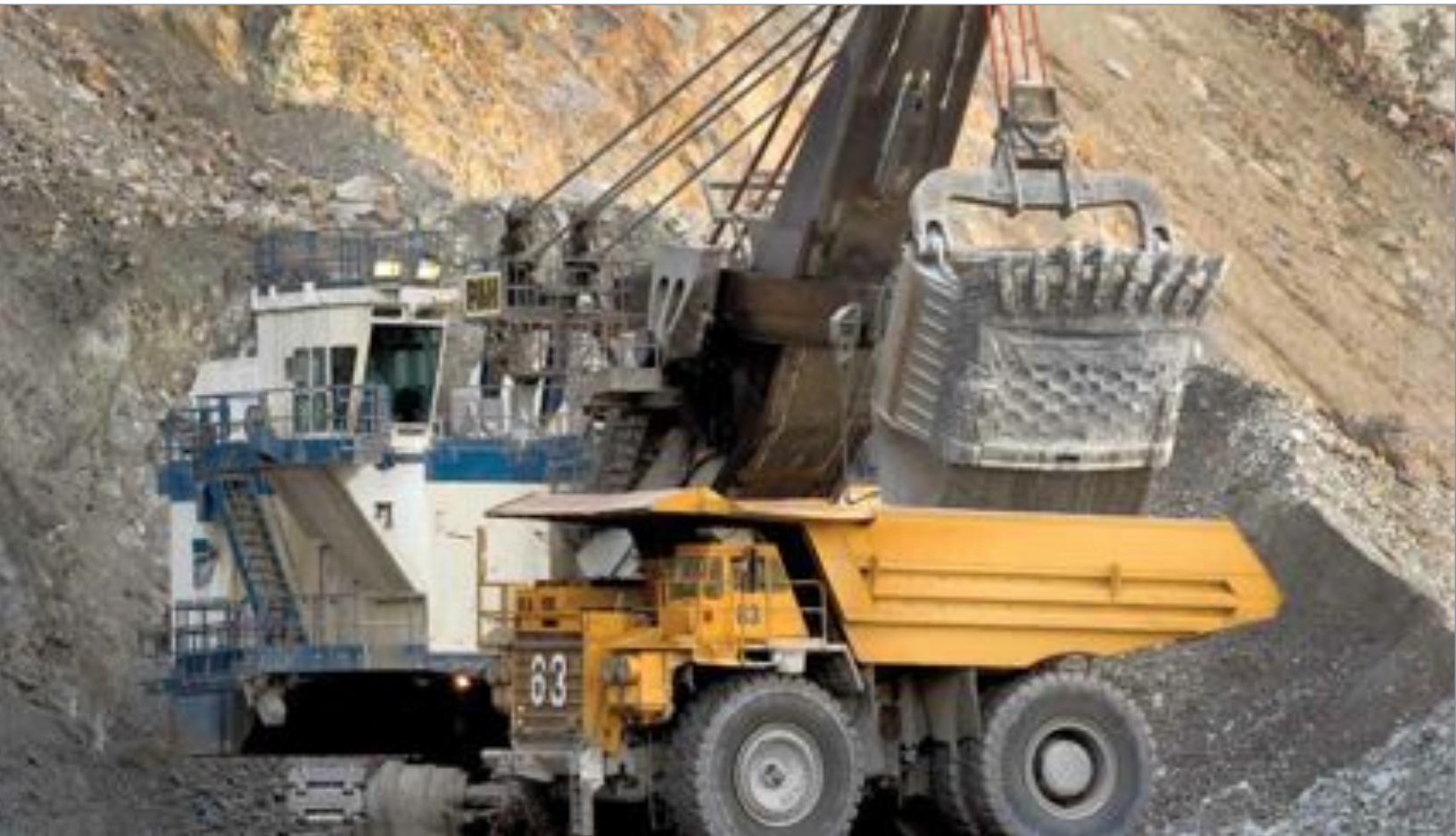
Electric shovel loading a haul truck at the Endako Mine
