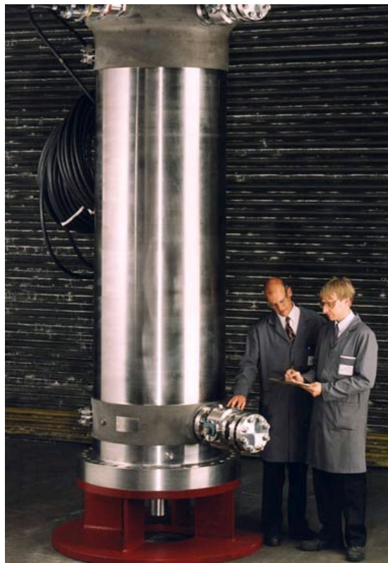
2,500kW, 9kV engineered variable speed deepwater subsea motor driving a multiphase pump in super duplex stainless steel.
