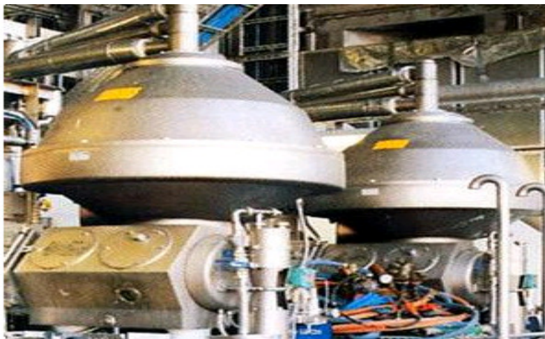
Centrifugal separators – Separators built of duplex stainless grades like 2205 (3% Mo) or 2507 (3-5% Mo) can be used for cleaning produced water.
