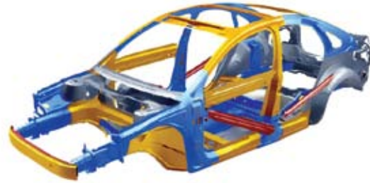
2008 General Motors “body-in-white” showing use of molybdenum-bearing high-strength steel
